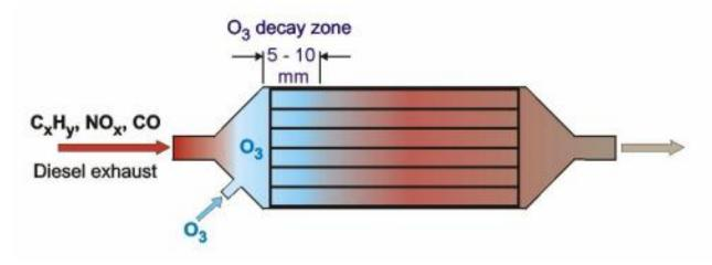
Under conventional implementation, when ozone is formed upstream the catalyst bed, the efficiency of ozone-catalytic process significantly decreases due to the parallel reaction of ozone decomposition to molecular oxygen - inactive at low temperatures
