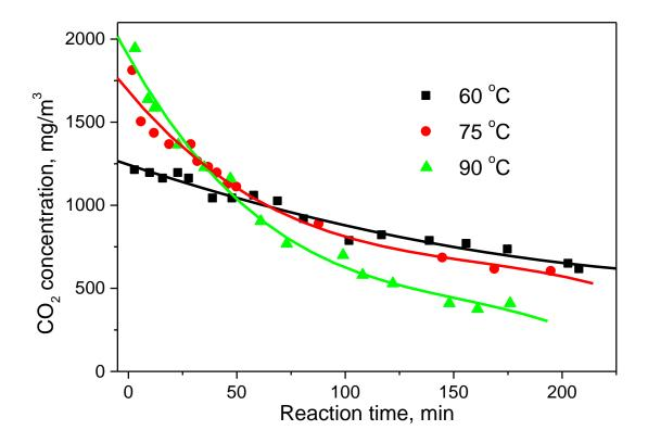
Regeneration of the 0.5% Pd/10%  $MnO_2/\gamma$ -Al<sub>2</sub>O<sub>3</sub> catalyst, containing 7.5 wt.%. CP, by ozone for 3 hours at 60- 90 C leads to the 1.3-1.5% weight loss.
