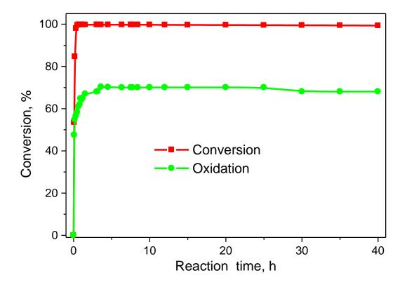
For the 0.5% Pd/10%  $MnO_2/\gamma$ -Al<sub>2</sub>O<sub>3</sub> catalyst, conversion of Toluene prevails over its oxidation. As a consequence, accumulation of the condensed products takes place on the catalyst surface.
